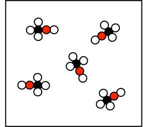
Because CH<sub>3</sub>OH does not dissociate in water there are no charged particles to carry a current
