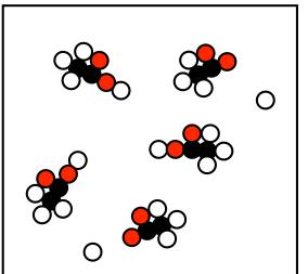
Because CH<sub>3</sub>COOH partially dissociates in water it contains a low concentration of current carrying charged particles
